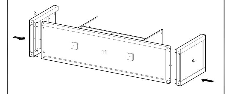
Attach panels (3,4) to bottom panel (11) using cam bolts and dowels as guides.
